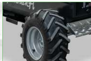
Deep tread rear tires with high blocks for better traction and grip
