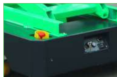
BDS operating panel, integrated in the chassis
