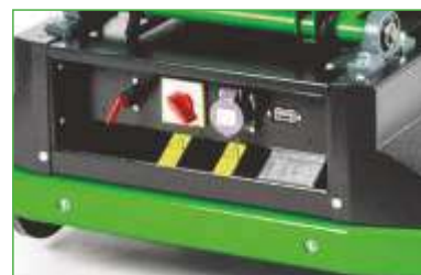
Extra operating panel integrated in chassis with battery indicator
