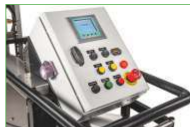
PLC controller from SIEMENS with touch panel
